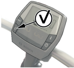
Image 21: Switching the display on and off
