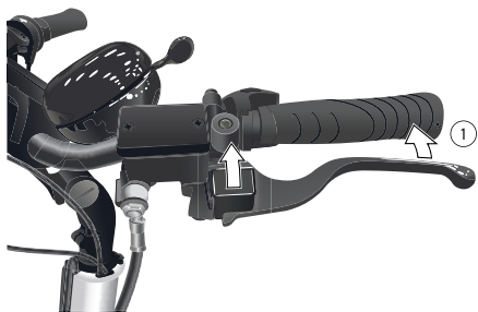
Image 23: Releasing the parking brake
