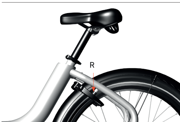
Image 38: Checking the lock rubbers
