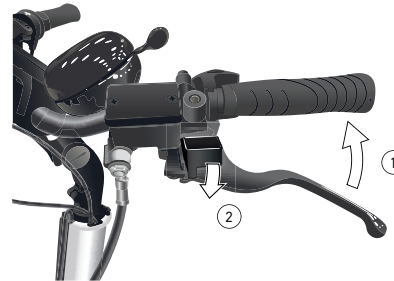
Image 22: Locking the parking brake
