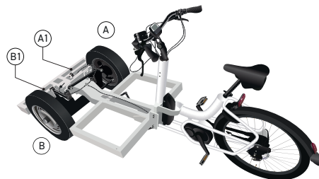
Image 32: Removing and placing a front tyre
