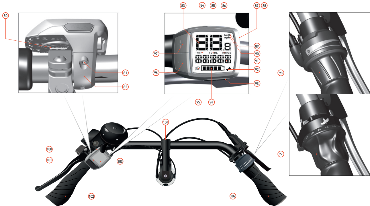
Image 4: Handlebar with Purion display and gearshifter without gear indicator (Rohloff/Enviolo)
