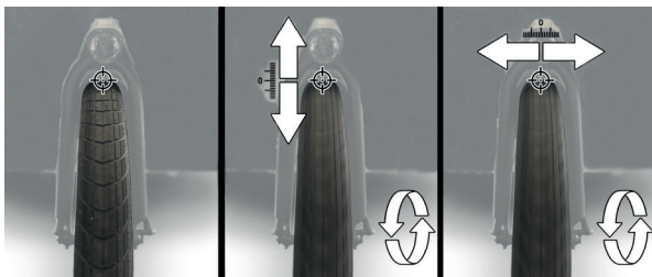
Image 34: Checking the rear wheel trueness
